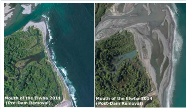
Mouth of the Elwha River, Washington, where dam removal has restored natural sediment flows. Photo: National Park Service
